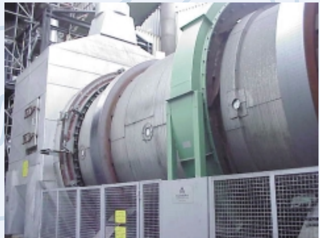
The Kumera steam dryer is the first one designed especially for the drying of abrasive materials.
