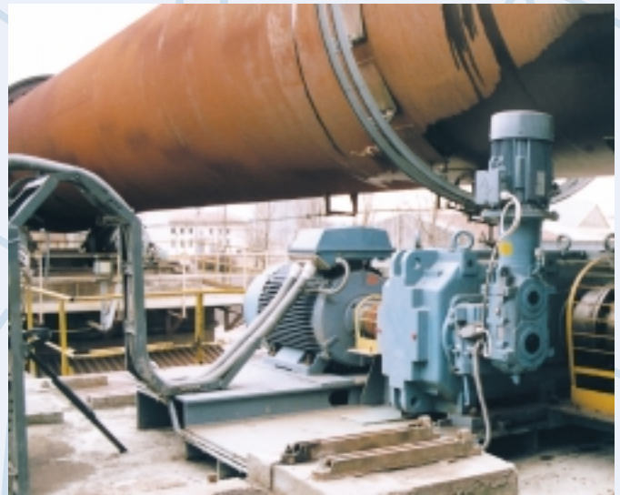
A drive unit with an auxiliary drive for a leca bebble dryer drum.
