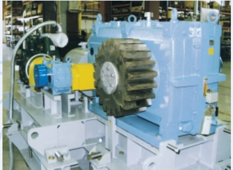
A drive unit complete with a segmental girth gear and an auxiliary diesel drive for a lime kiln on test run at the workshop, to be shipped to China.
